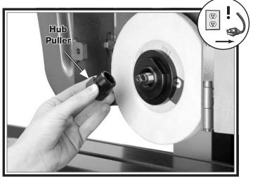
Figure 32. Hub puller installation.
